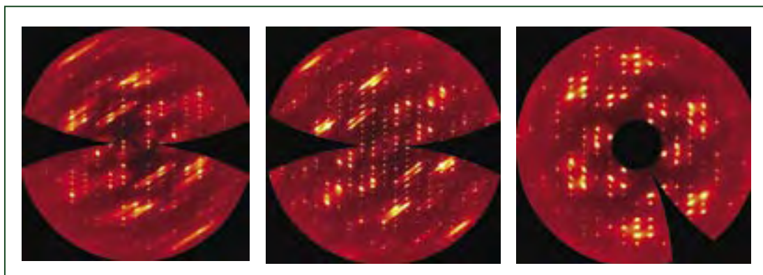
From left to right, the ( h 0 l ) sections of the three polymorphs I, II and III of MeMe.
