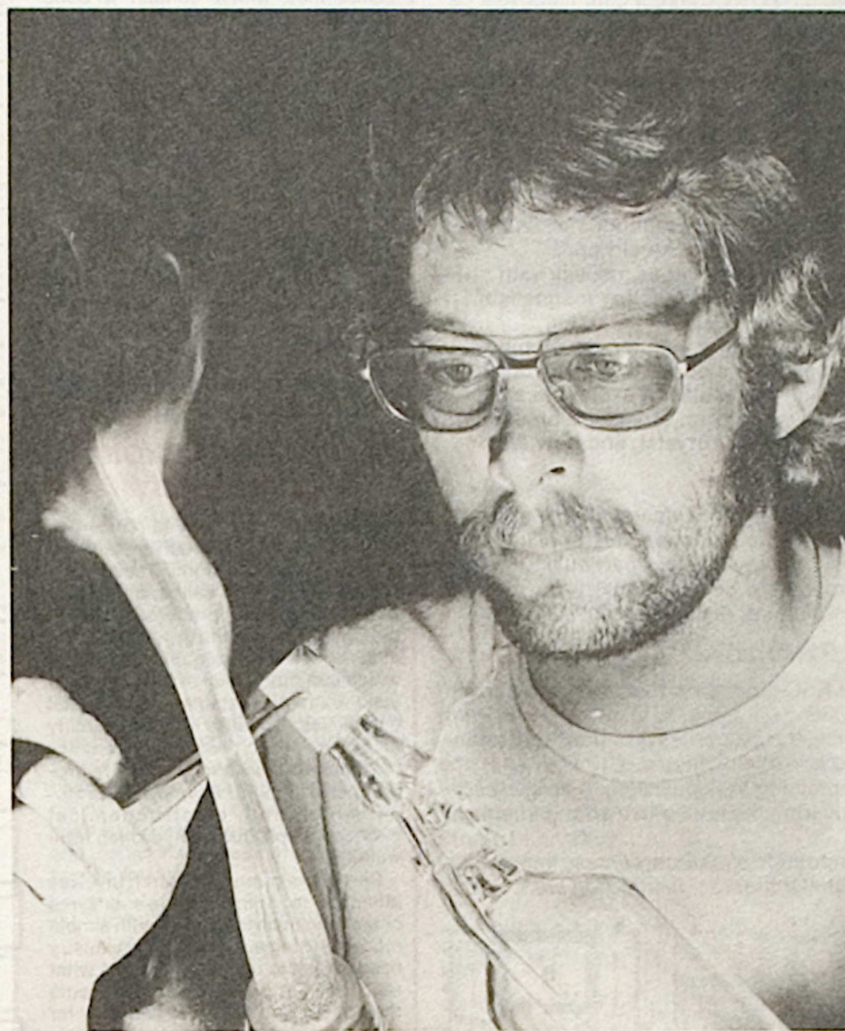
Mr Chris Tomkins, one of the two scientific glassblowers in the School, at work constructing a piece of the complex apparatus that is not commercially available and which has to be made.
