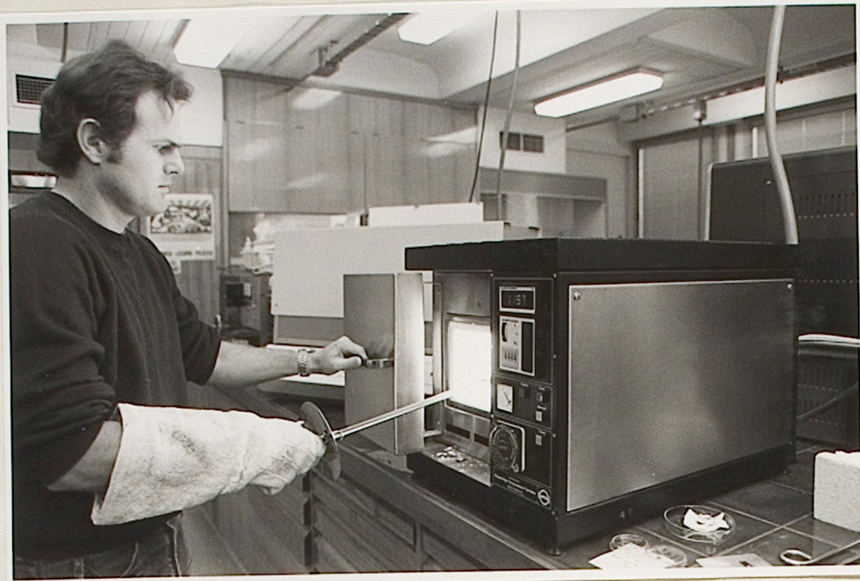
MR. PETER BARLOW UNLOADING A HIGH TEMP. FURNACE USED FOR GROWING CRYSTALS STUDIED AT ATOMIC RESOLUTION BY THE SOLID STATE GROUP.
